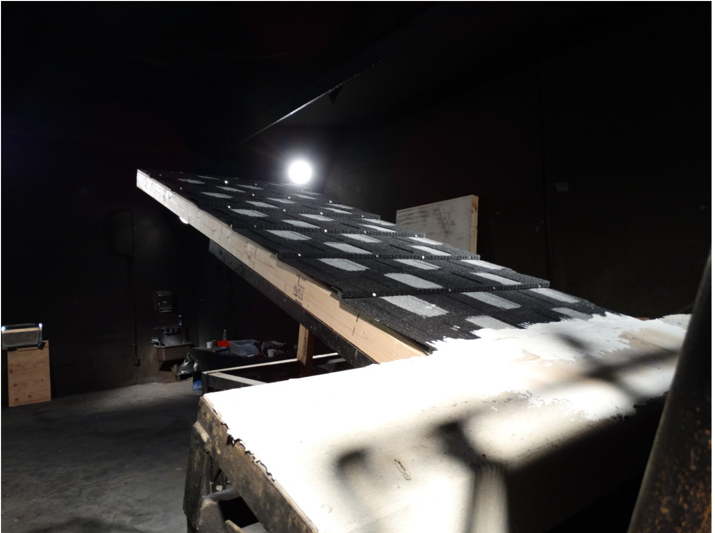
Photo 3: Spread of flame Test deck assembly from the top.
