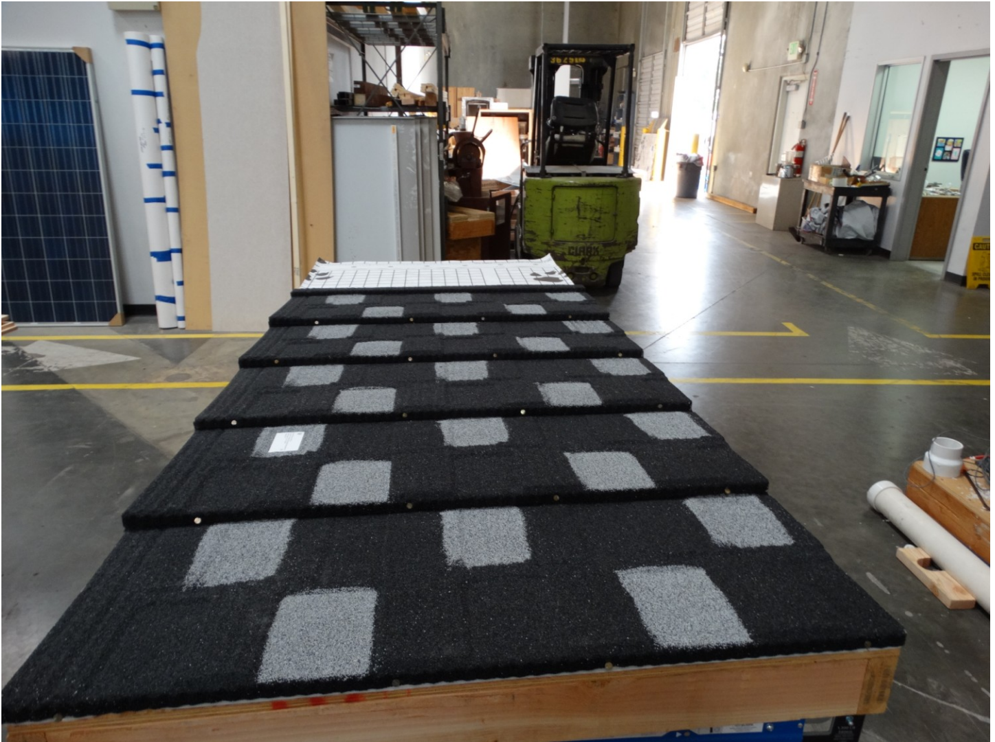
Photo 2: (Tefute Stone Coated Roofing System) Spread of Flame test deck assembly.
