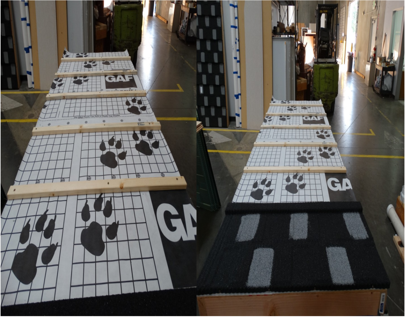
Photo 1: Spread of Flame test deck assembly with Tigerpaw Underlayment.
